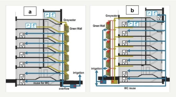
Figure 4: Possible implementation schemes for greywater collection, treatment, and reuse in the same building with green walls: a) floor-by-floor and b) unified.
