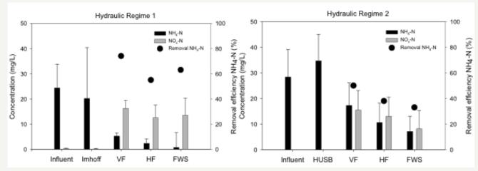
Figure 4. Mean concentrations of NH<sub>4</sub>-N, NO<sub>x</sub>-N, and NH<sub>4</sub>-N removal for each constructed wetland, for the hydraulic regimes 1 and 2 (adapted from Ávila et al. (2013, 2016).
